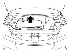
2. Remove the battery cover from its front side.
